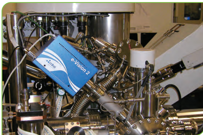
e-Vision 2 in use as a troubleshooting tool on vacuum-based surface analysis equipment.
